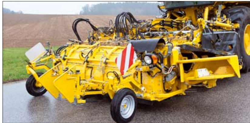
PASWh-Schlegler, Schleglerklappe oben
